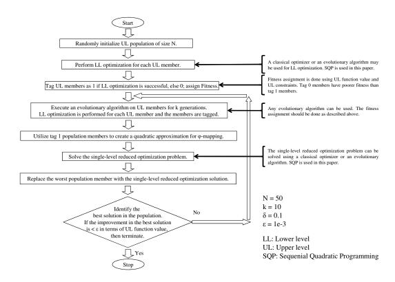
Figure 1: Flowchart for incorporating approximated  $\varphi$ -mapping in an evolutionary algorithm.
