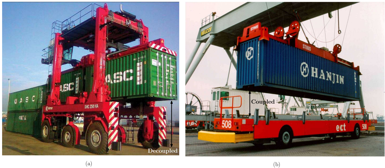
Figure 1 a) Automated Lift Vehicle (ALV) (source: www.sae.org ), b) Automated Guided Vehicle (AGV)
