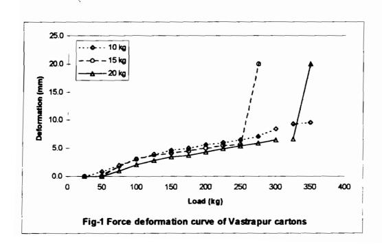
When the three cartons are loaded up to their respective stacking strength, the deformation does not exceed 10 mm (figure 1). This is satisfactory.
